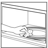
sudsy water and a sponge or soft cloth. Use only mild, nonabrasive soaps or a mild detergent. Be sure to keep the areas clean where the door and oven frame touch when closed. Wipe well with clean water. Over time, stains can occur
