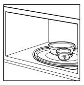
To test a dish for safe use, put it into the oven with a cup of water beside it. Cook at 100% cook power for 1 minute. If the dish gets hot and water stays cool, do not use it.
