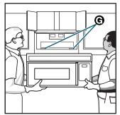
microwave oven downward. (Be careful that door does not swing open.) Lift off the support tabs **(G)** at the bottom of the mounting plate. Set the microwave oven aside on a protected surface.
