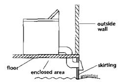
The exhaust vent must be securely fastened to a non-combustible portion of the mobile home structure and must not terminate beneath the mobile home.
