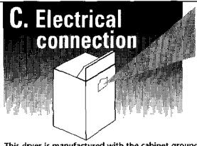
This dryer is manufactured with the cabinet-ground conductor connected to the NEUTRAL (center) of the wiring harness at the terminal block. If local codes do NOT permit this type of connection, use "Four-wire connection" instructions.
