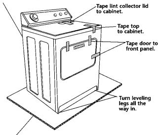
Slide dryer onto cardboard or hardboard before moving it across the floor to prevent damaging floor covering.
