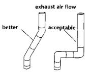
Select the route that will provide the straightest and most direct path outdoors. Plan the installation to use the fewest number of elbows and turns. Avoid making 90° turns.
