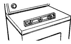
Check levelness of dryer by placing a level on top of dryer, first side to side, then front to back. If dryer is not level, adjust dryer legs up or down.
