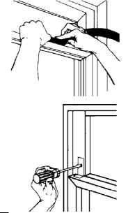
Insert window rail seal behind the top of the lower window sash and against the glass of the upper window. Place window-lock bracket on top of lower window and against upper window sash. Use a 2mm (3/32") drill bit to drill a starter hole through the hole in the bracket. Attach window-lock bracket. Seal small openings around window with gum-type sealer.
