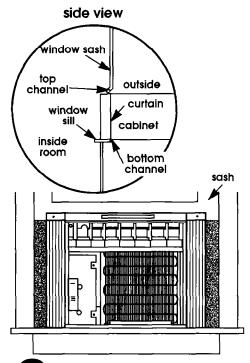
Place air conditioner in center of window. Lower sash (window frame) to hold cabinet in place.
