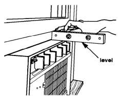
Place level on the top right edge of the cabinet. There should be a tilt to the outside of about one-half bubble. Place the level on the left side and check.
