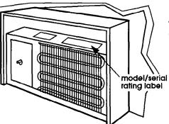
Specific electrical requirements are listed in the chart. Follow the requirements for the rating listed on the model/serial rating label.
