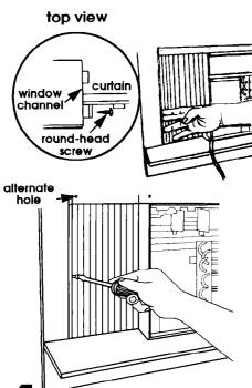
Pull curtain out until it fits into the window channel. Insert one of the round-head screws through curtain and into the window channel or through alternate hole at the top of the curtain and into the window channel to fasten the curtain to the window.
