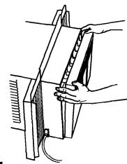
Push down on front panel and pull panel towards you to remove from cabinet.
