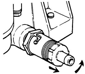
ROTATE PLUG COUNTER CLOCKWISE THEN PULL OUT TO DRAIN OIL
