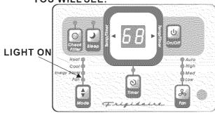
NOTE: Use this function only when cooling is not desired, such as for room air circulation or to exhaust stale air. (Remember to open vent during this function, but keep it closed during cooling for maximum cooling efficiency.) You can choose any fan speed
