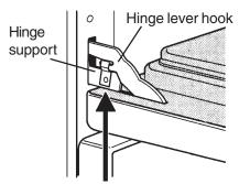
Lock engaged for door removal Figure 1
