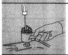
**6** ■ Pull up on spout body to keep tension on spout mounting bracket and nut. Tighten screw inside the spout until spout is securely in position. **Do not overtighten.** Snap on On/Off Cap.
