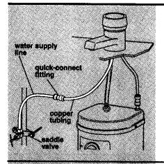
13 Connect water supply line from saddle valve to spout copper tubing with the factory-assembled quick-connect fitting. Push water supply line tubing straight into fitting as far as it will go. Pull on tubing.
