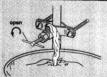
12. Slowly open saddle valve and flush line into bucket to remove any foreign material that may have been trapped in the supply line during saddle valve installation.
