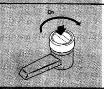
15 Push down and turn the On/Off Cap clockwise to open spout. Hold cap open to fill tank (about 1 minute). When tank is full, water will flow from spout. Release cap.
