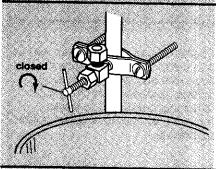
11 Turn saddle valve handle clockwise () until lance pierces soft copper tubing and valve is firmly seated. If the water line is not copper, turn the saddle valve handle clockwise until the valve is firmly seated. The valve is now in the closed position.
