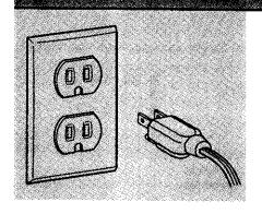
16. Plug power supply cord into grounded outlet.
