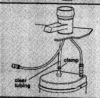
9. Connect clear tubing from spout to center tank tubing using clamp. Make sure clear tubing does not kink.
