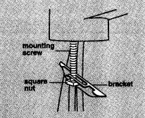
5 Loosen square nut until it is flush with end of the mounting screw. Tip spout bracket against mounting screw. (Bracket will form a "y" when in the correct position.)
