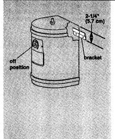
■ Position tank vertically beneath spout so that clear tubing from spout reaches center stainless tubing on tank, and tank touches wall. Use a pencil to mark on the wall where the top of tank needs to be located. Set tank aside. Mark a second line 2-1/4" (5.7 cm) below the first line.
