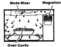
A magnetron in the microwave oven produces microwaves. The microwaves move into the oven where they are scattered or stirred by a mode mixer (like a fan). Microwaves bounce off metal oven walls and are absorbed by food.
