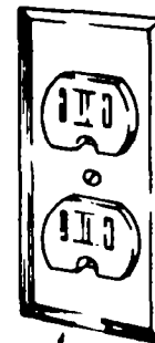
3-PRONG/ GROUNDING TYPE WALL RECEPTACLE
