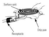
To remove the surface unit, lift it about 1 inch above the drip pan and pull it out.
