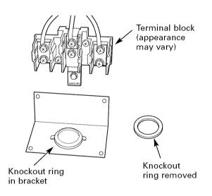
The power cord installations only (see the next step if using conduit), assemble the strain relief in the hole. Insert the power cord through the strain relief and tighten. Allow enough slack to easily attach the cord terminals to the terminal block. If tabs are present at the end of the winged strain relief, they can be removed for better fit.
