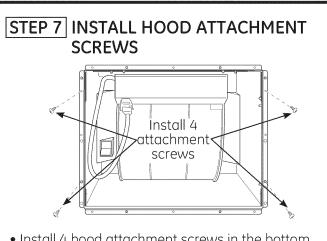
• Install 4 hood attachment screws in the bottom of the support as shown. Leave 1/4" gap between screw head and support flange.
