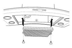
• Install the black charcoal filter into the center opening. Secure the filter with thumbscrews on each side.
