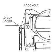
• Secure the house wiring to the junction box with a strain relief.
