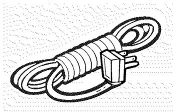
The use of an extension cord is not recommended. However, if an extension cord is required to reach the nearest wall receptacle, use only a UL-listed, 3-wire, grounded, 14 gauge, 15A, 125V appliance extension cord.
