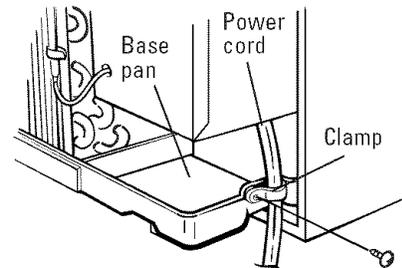
6 When the wall outlet is to the left, extend the cord under the unit and hold it in place with the clamp.
