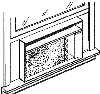
4 Reinstall the locking plate with the tab behind the wall case flange. Tighten the screw.
