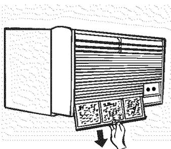
Replace the clean filter by pushing it back into place.
