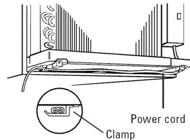
7 Attach the front grille. An opening for the power cord is on the bottom of the front grille.
