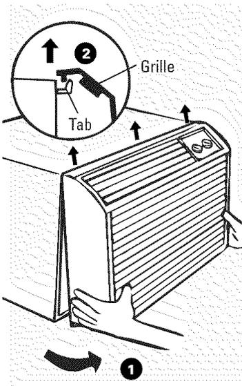
The front grille can be removed for more thorough cleaning or to make the model and serial numbers accessible.
