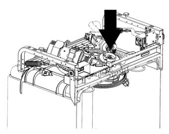
Once the sump is removed, the dishwasher can be tipped to correct position to complete repairs.
