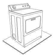
**1.** Open dryer door and remove drying rack, if included. Wipe drum with damp cloth to remove any dust.
