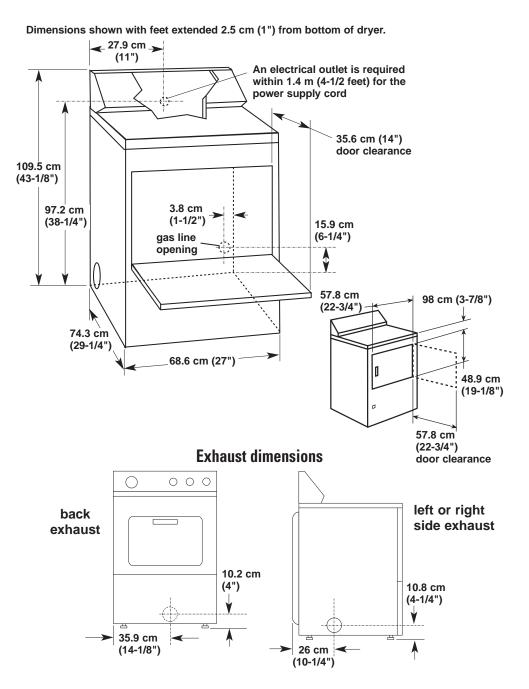
• **Spacing:** Keep a minimum distance of 10 cm (4 inches) between the rear of the dryer and any wall, a minimum distance of 2.5 cm (1 inch) at the sides, and a minimum distance of 46 cm (18 inches) to any cupboards above the dryer. The minimum distance in front of the dryer should be sufficient to allow the door to fully open.
