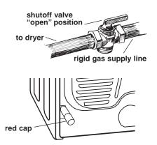
The dryer gas inlet connection is a 3/8" NPT thread. An adapter is supplied for conversion to standard ISO.228-1 thread (3/8" BSP).
