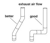
When using elbows or making turns, allow as much room as possible. Bend vent gradually to avoid kinking.
