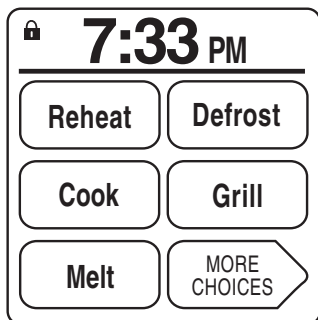
Display with padlock in upper, left-hand corner. Child Lock active.
