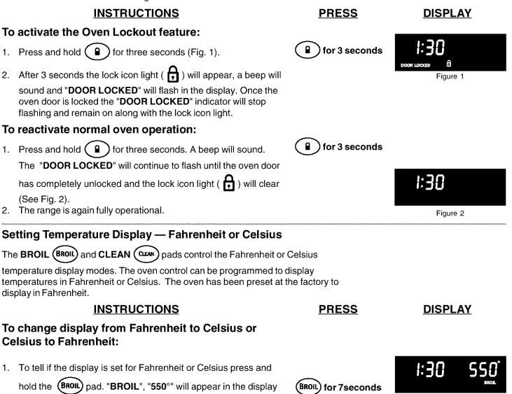
(See Fig. 3) and continue to HOLD for 7 seconds. A beep will then sound. If "**F**" appears, the display is set to show temperatures in Fahrenheit (Fig. 4). If "**C**" appears, the display is set to show temperatures in Celsius (Fig. 5).
