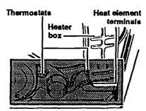
Electric dryer with back panel removed
