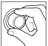
Signal selector is part of the Start button. Set the Cycle Signal selector to On if you want the dryer to sound a signal when a cycle is finished. The signal is helpful when you are drying permanent press, synthetics, and other items that should be removed from the
