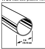
Use 4 in (10.16 cm) heavy metal or flexible metal vent. Do not kink or crush flexible metal vent. It must be completely extended to allow adequate exhaust air to flow. Check vent after installation. Refer to your Installation Instructions for proper
