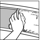
rinse or wash screen to remove lint. Wet lint is hard to remove.
