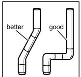
the exhaust vent. Avoid 90° turns, if possible. Allow room when using elbows or making turns. Bend vent gradually to avoid kinking.
