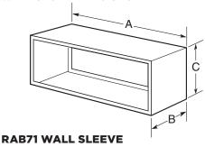
Heavy-gauge galvanized steel, with insulation. A -42", B -13-3/4", C -16"
