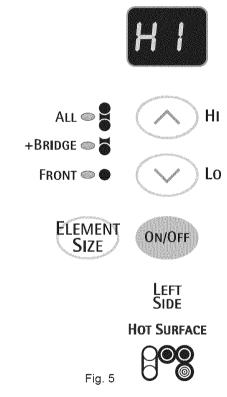
NOTE: If all 3 Bridge elements are selected, any previous power level setting for the LEFT REAR element will be changed to the power level setting for the Bridge.
