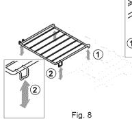
The Flat Half Rack has a removable insert that can provide extra space for larger food items. The right half rack portion may still be used for other food items like a casserole dish (See Fig. 5). To remove the insert, squeeze on the left front insert side (See Fig. 7) of the rack and tilt out clockwise. To reinstall insert rear hooks at back of insert (See 1-Fig. 8) and lay insert down. Make sure both insert front hooks snap into rack (See 2-Fig. 8).
