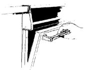
During broking the oven door must be partly open. A built-in stop will hold it there
