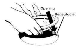
**2.** Line up opening in the reflector bowl with the surface unit receptacle.
