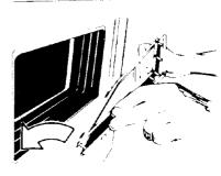
Fit the bottom labs of the frame into the bottom of the window opening
