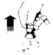
SURFACE UNITS AND **REFLECTOR BOWLS** REMOVING
